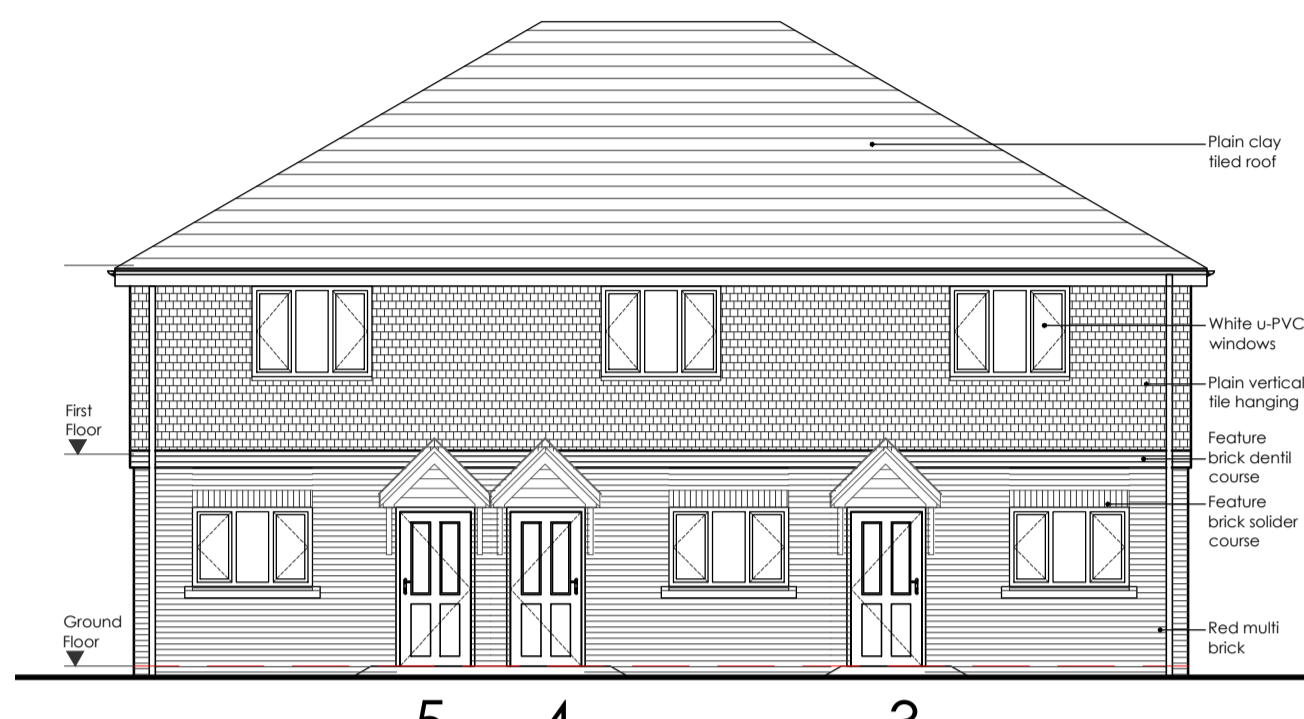
Front Elevation (West)
